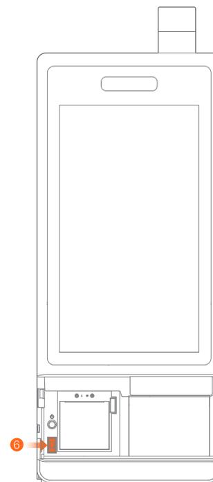
6 Press the power switch to turn on the host.
