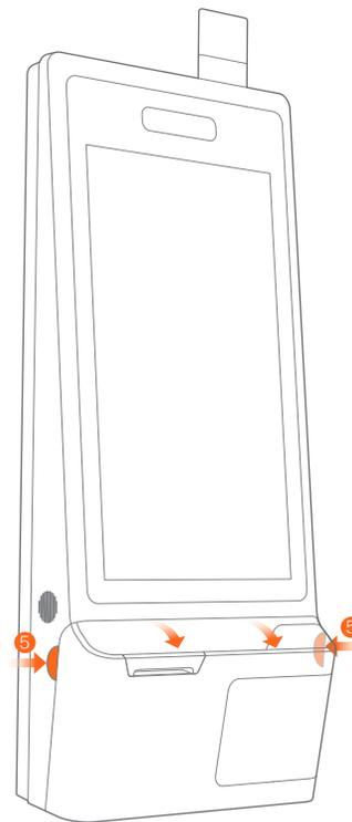
5 Press the buttons on both side of the host at the same time to open the flip panel.
